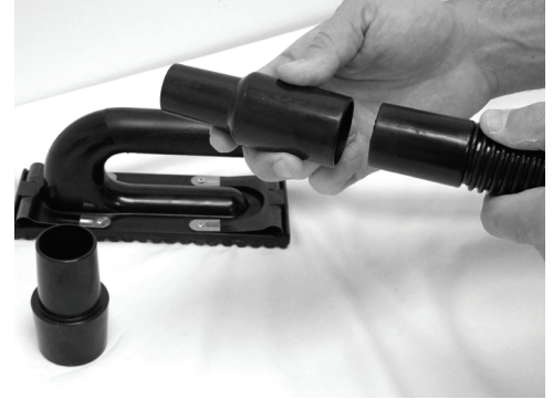
Attach hose adapter to opposite of hose. Use correct size adapter to fit your vacuum
