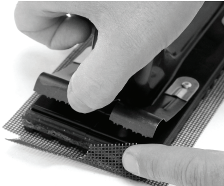
Lift front and back clips and insert sandscreen onto sanding head
