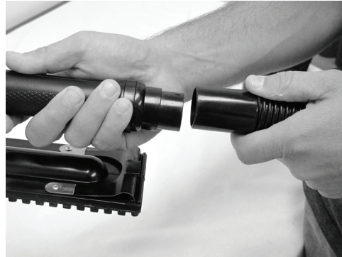
Attach supplied flexible hose onto sanding head
